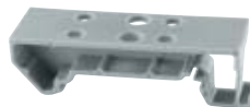
58 x 18 x 18 mm mounting base for panel mount terminals on DIN 35 rails. (Hole dia 4.3 - 4 Nos & 5.5 - 2 Nos)
